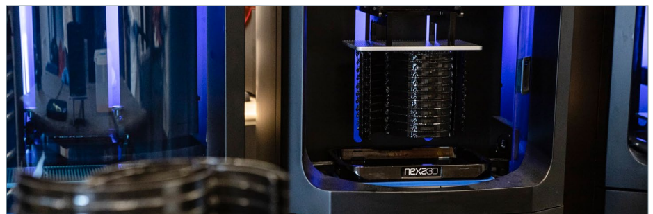
Face shield frames being produced on a Nexa3D NXE400 3D printer
