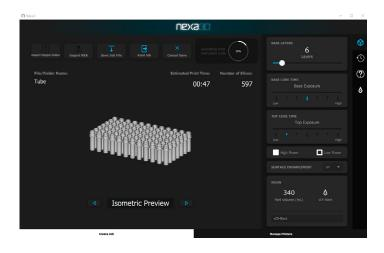
of PA6GF15 material. For this specific part we used xCE-Black material which has excellent mechanical properties and high temperature resistance, as this was the customer's requirement. The main benefit of 3D printing in this case is the tooling cost, which is zero, thus lifetime project cost is smaller than in the case of injection molding."
