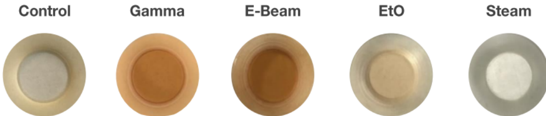
Color samples before and after sterilization
