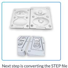
into a mold design which is done by inverting the part into a cavity, in a block of material, and then adding the inlet gate(s) and initial venting. The 2-part initial design allows for
