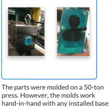
molding unit. An aluminum mold frame was used to hold the assembled mold, cycle time per part was around 5 minutes, and 1 minute
