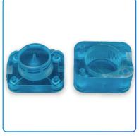
The molds were printed at a 100µm resolution to ensure good mold quality while optimizing the build for fast production.
