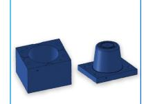
After the design is completed, the digital design (STEP file) in converted into a mold design which is done by inverting the part into a cavity, in a block of material, and then adding the inlet gate(s) and initial venting.
