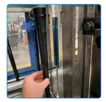
In this specific case the split mold allowed for manual demolding, meaning no part of the mold to had get dissolved, as the part could be pulled off.
