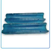
The molds were printed at a 76.5µm resolution to ensure good mold quality while optimizing the build for fast production.
