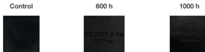
Effect of UV exposure on color of the specimens
