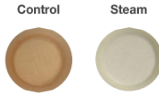
Color samples before and after sterilization (with non-dyed version of xPRO1100)
